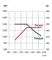
9-litre, 320 hp Biodiesel, HVO, diesel
