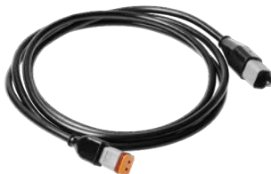
ADR cable harness RKKIB 2x1.5 mm 2 extension cable. 1 DT female 2 pol + 2 m cable ending with DT male 2 pole connectors. Part no. 2786411
