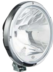
Hella Rallye 3003, pencil beam, clear lens, Ref. 50 Hella Halogen spot lamp, 222 mm. Black plastic housing with chrome trimring. Real, clear glass lens, pencil beam. H1 bulb, not included. Recommended H1 HD premium replacement bulb: Scania part no. 1905134. Part no. 2060523
