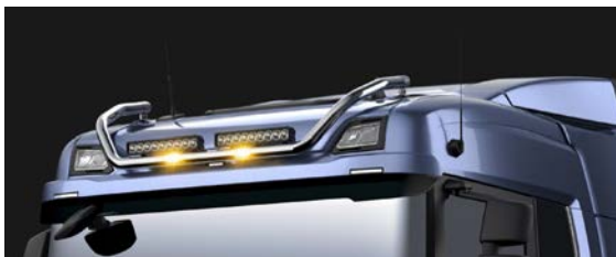
Scania light bar for normal roof, short with LED strobe flashers Polished 60 mm stainless steel roof light bar. Short version, with 2 strobe flasher LEDs, for normal roof. Pre-wired and fixed brackets for 4 aux lamps (lamps are not included). Part no. 2706266
