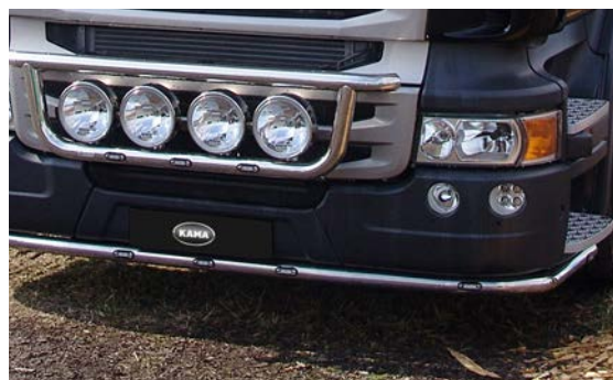
Front pipe with LED, G- and R-series low bumper m/y 2014– As part no. 2203831 with 5 white front-facing LED modules + 1 orange LED module on each side. Part no. 2387162
