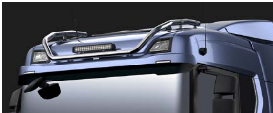
Scania roof light bar for normal roof, long without LED Polished 60 mm stainless steel light bar. Long version, without styling LEDs for normal roof. Pre-wired and fixed brackets for 4 aux lamps (lamps are not included). Part no. 2706263
