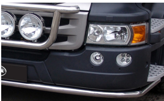
PGR-series, low bumper m/y 2004– Styling pipes in polished stainless steel, without LED's. Part no. 2396049
