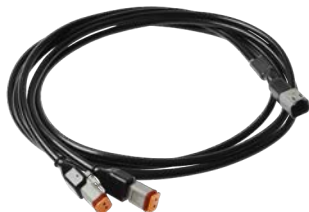
ADR cable harness RKKIB 2x1.5 mm 2 branch cable. 1 DT male 2 pol + 1.1 + 2.5 m cable ending with 2 DT female 2 pole connectors. Part no. 2786413
