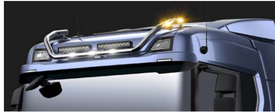
Scania light bar for normal roof, short with LED Polished 60 mm stainless steel roof light bar. Short version, with styling LEDs for normal roof. Pre-wired and fixed brackets for 4 aux lamps (lamps are not included). Part no. 2706264
