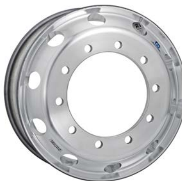
Aluminium rim, Dura Bright Dura Bright is a patented surface treatment allowing easy cleaning with soap and water. These wheels do not need polishing. 22.5x8.25. Part no. 2294371 22.5x9.00. Part no. 2294372 22.5x11.75. Part no. 2294373
