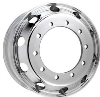
Aluminium rim, Dura Bright Dura Bright is a patented surface treatment allowing easy cleaning with soap and water. These wheels do not need polishing. 22.5x8.25. Part no. 2294371 22.5x9.00. Part no. 2294372 22.5x11.75. Part no. 2294373
