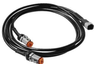
ADR cable harness RKKIB 2x1.5 mm 2 + 2x1 mm 2 branch cable. 1 DT male 4 pol + 1.1 + 2.5 m cable ending with 2 DT female 4 pole connectors. Part no. 2786415
