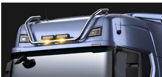
Scania light bar for high roof, short with LED strobe flashers Polished 60 mm stainless steel roof light bar. Short version, with 2 strobe flasher LEDs, for high roof. Pre-wired and fixed brackets for 4 aux lamps (lamps are not included). Part no. 2706260
