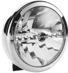
Cibié Super Oscar, 230 mm, LED, broad beam, LED position lights, chrome, Ref. 27.5 Full LED spot lamp, chromed alu housing and trim ring, clear plastic lens, IP67, 12 V/24 V. Part no. 2447400
