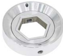
DrainBlank “DrainBlank” protects against theft of fuel through the existing drain plug beneath the tank. It has been designed to fit over the existing fuel tank drain plug. The outer ring rotates freely and cannot be removed. Part no. 2375264
