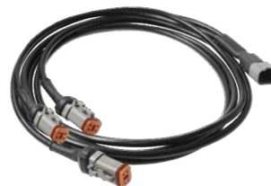
ADR cable harness RKKIB 2x1.0 mm 2 branch cable. 1 DT male 2 pol + 1.1 + 2.5 m + one extra loop with 2,2 m cable. ending with 1x3 DT female 2 pole connectors. Part no. 2786414
