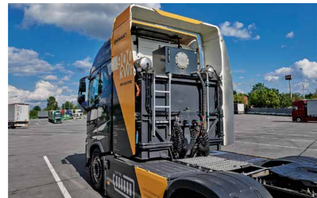
Designwerk places two of the four battery packs in the tower behind the cab
