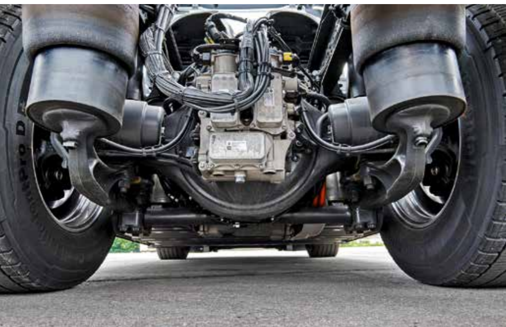
E-axle with two electric motors plus automated four-speed gearbox
