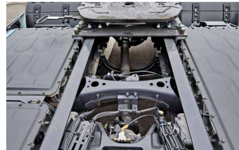
Six-speed (or rather, five-speed) gearbox with flange-mounted cardan shaft
