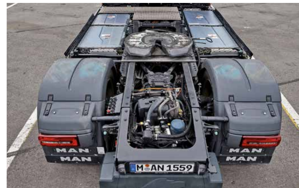
The cardan shaft limits space, so the eTGX has a maximum of 534 kWh on-board
