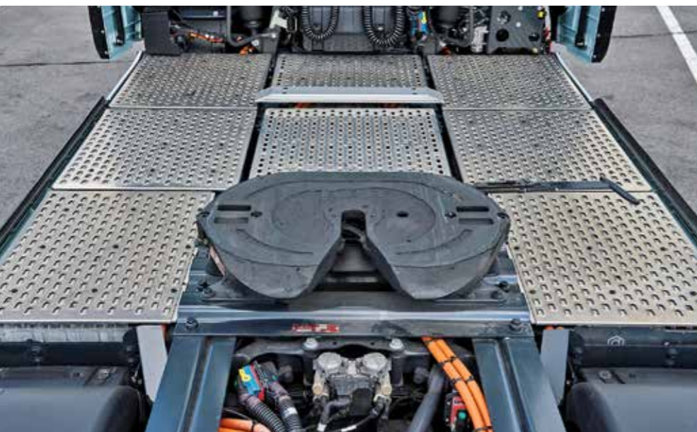
Thanks to the electric axle, the Iveco can store 738 kWh of gross power in nine battery packs
