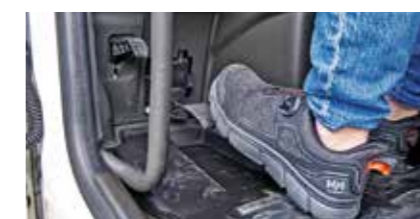
Top: Infinitely adjustable recuperation by pedal
