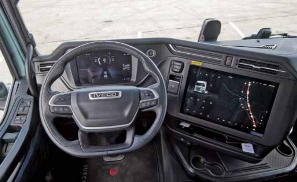
Iveco places the huge 17-inch screen in the centre console too low
