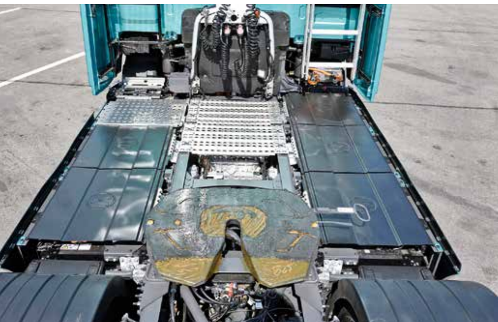
With a net battery capacity of 421 kWh, the Volvo lags well behind
