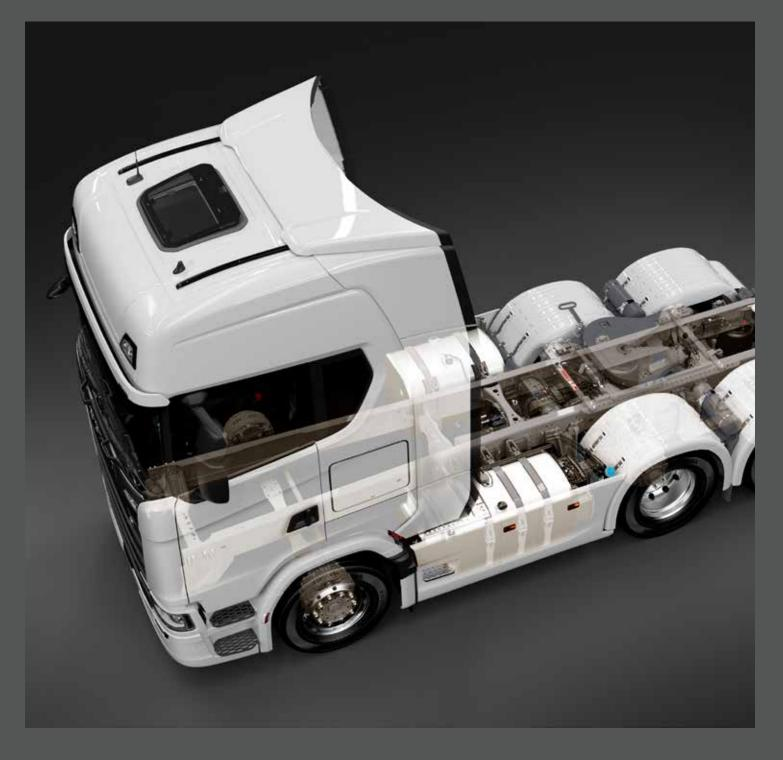
Components can now be mounted both from the front and rear axle, facilitating a more versatile bodybuilding process.
