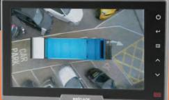
This exciting new development provides drivers with a single clear view image of all near-field blind spots around the vehicle – which is a massive leap forward in vehicle safety!
