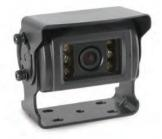
**BE-800C** - PAL GB9091069 BE-800C(40) - Narrow viewing angle: 33 x 25 x 40° PAL GB9091066 BE-800C(78) - Narrow viewing angle: 64 x 47 x 78° PAL GB9091064 - Waterproof to IP69K, No audio PAL GB9091103 **BE-850C** - 12/24Vdc Waterproof to IP69K PAL GB9091195 **BE-801C** - NTSC GB9091079 BE-801C(40) - Narrow viewing angle: 33 x 25 x 40° NTSC GB9091085 BE-801C(78) - Narrow viewing angle: 64 x 47 x 78° NTSC GB9091084
