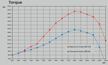
**Test conditions.** Air temperature 25°C. Barometric pressure 100 kPa (750 mmHg). Humidity 30%. Diesel fuel acc.to ECE R 24 Annex 6. Density of fuel 0.84 kg/dm³. Viscosity of fuel 3.0 cSt at 40°C. Energy value 42,700 kJ/kg. **Power test code** ISO 3046. Power and fuel values ±3%.
