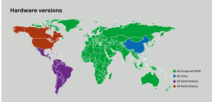
There are four different hardware versions depending on the network standard in the world. Hardware version should be selected based on the final destination of the engine.
